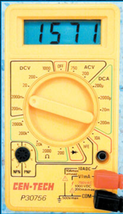
13. The same AA battery when read from the 2000m (2 DCV) scale.
